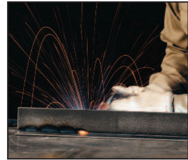
STT® using CO 2 and .045 in. solid wire. Note reduced spatter and fume.
